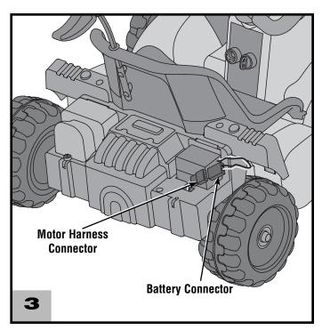
• Plug the battery connector into the motor harness connector. **Note:** If the battery connector will not plug into the motor harness connector, turn it over and try again. Do not force the battery connector into the motor harness connector.
